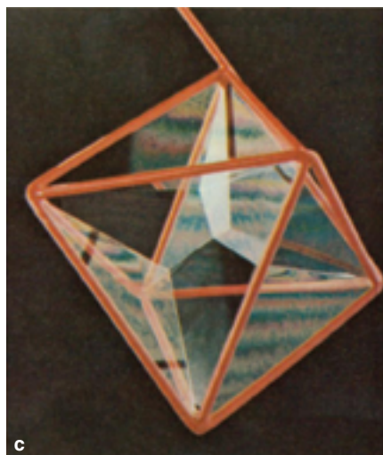
Figure 7. Soap films can be used to find the minimum surfaces for three-dimensional problems. a . Tetrahedron. b . Cube. c . Highest symmetry for an octahedron. d . Octahedron with a "square"-shaped surface in the center.
