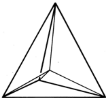
Figure 6. This diagram of the minimum surface formed by a tetrahedron reveals a plane that is hidden in the photograph 7a.
