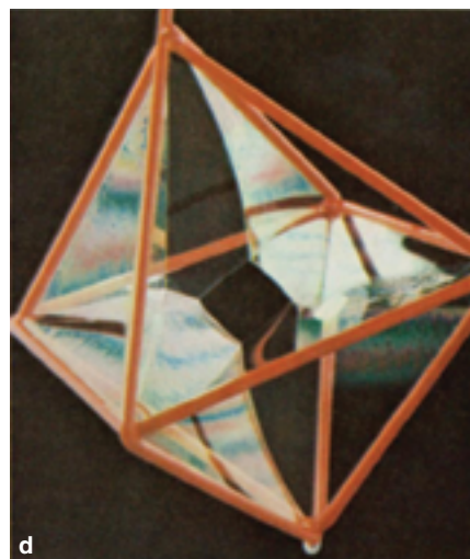
Figure 7. Soap films can be used to find the minimum surfaces for three-dimensional problems. a . Tetrahedron. b . Cube. c . Highest symmetry for an octahedron. d . Octahedron with a "square"-shaped surface in the center.
